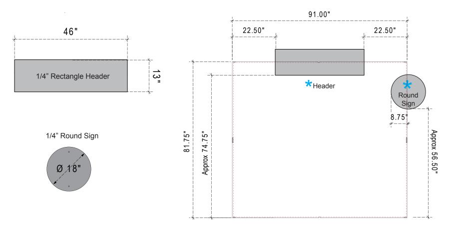
**NOTE:** When using headers with the Sacagawea unit a portion of the graphic will be covered. Please design graphic layout according to desired header shape and location.\*
